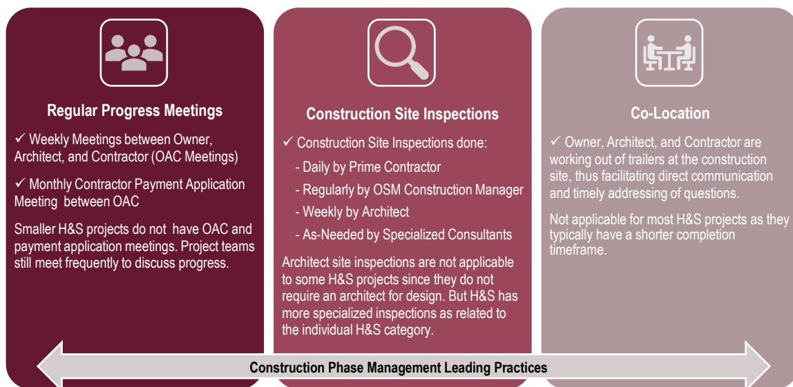
EXHIBIT 11. CONSTRUCTION PRACTICES EMPLOYED AT MADISON HIGH SCHOOL, KELLOGG MIDDLE SCHOOL, AND H&S PROJECTS
